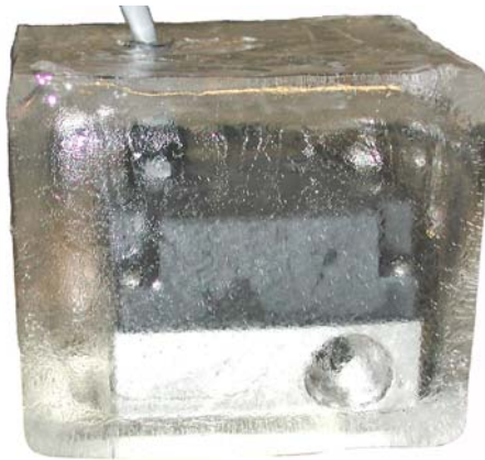
LT800 Series flowmeter – still functioning in a block of ice
