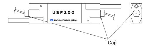
The cap is tightened at specified torque. Never turn the cap.
